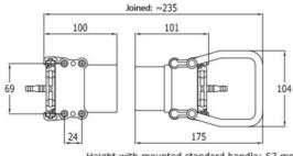
Height with mounted standard handle: 57 mm. Height with mounted flat handle: 40,5 mm.
